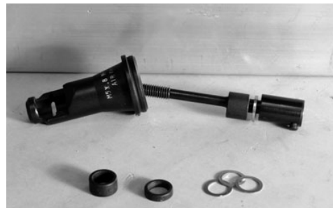
Front end assembly with longest spacer to suit 1.0D insert and shim washer.
