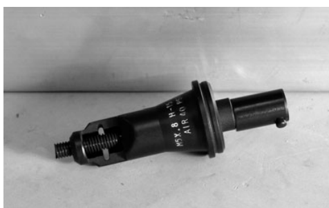
Finished front end assembly with mandrel wound through the pre-winder nozzle.
