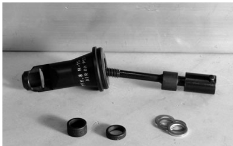
Front end assembly with longest spacer to suit 1.0D insert.
