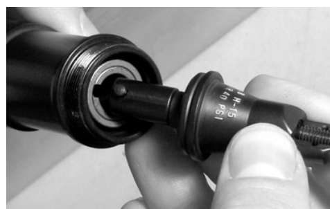
Locate mandrel pin in the slot of the driving spline and slide the front end assembly into the case.
