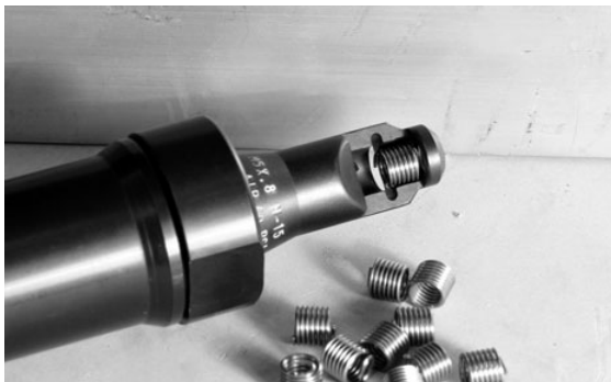
Place wire thread insert into chamber and ensure the tang end is facing down (nearest the nose end).
