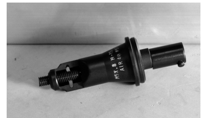
Finished front end assembly with mandrel wound through the pre-winder nozzle.
