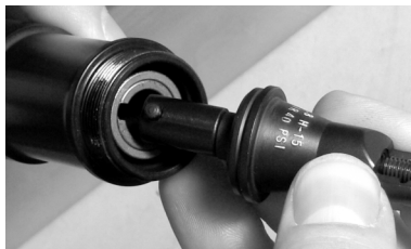
Locate mandrel pin in the slot of the driving spline and slide the front end assembly into the case.
