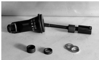
Front end assembly with longest spacer to suit 1.0D insert.
