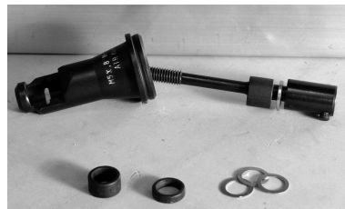
Front end assembly with longest spacer to suit 1.0D insert and shim washer.
